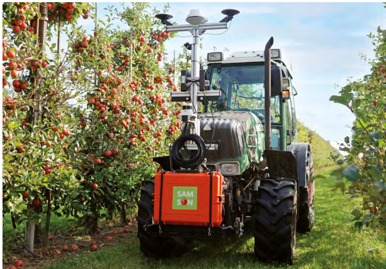
The sensor box developed as part of the SAMSON project, which is used to collect and process data in orchards, can be mounted on any tractor.
